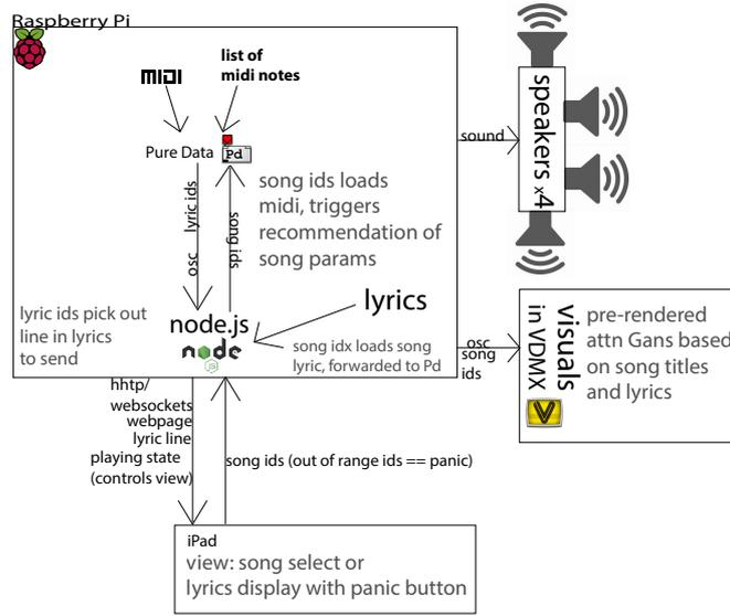
Fig. 4: I/O diagram for the KoD's system setup
